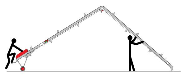
**4.** With man 2 supporting the machine at centre, (fig 3). Man 1 releases the brakes and walks the base backwards until the machine is fully open.
