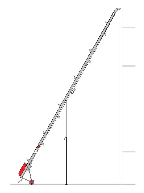
**10.** When machine is erect, place first load onto loading hoop. Centralise loading guides and tighten to minimise un-even loading.
