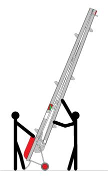
**3.** Release anti-luce catches and walk top boom approximately 5-6 paces away, then rest head of machine on the ground. (fig 2)
