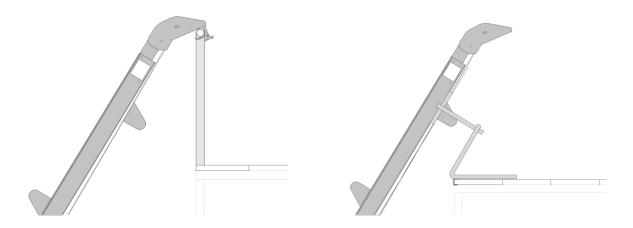
**8.** With the machine secured on to the scaffold. The delivery chute is now fitted by slotting in to the head lugs. Then rotate and extend as required. (Fig. 7.)
