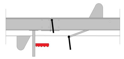
**6.** The head of the machine is now ready to be raised on to the roof/ scaffold by block and tackle or rope. Ensure lifting device is secure and safe. The base is guided and positioned by man 1. (fig. 4)
