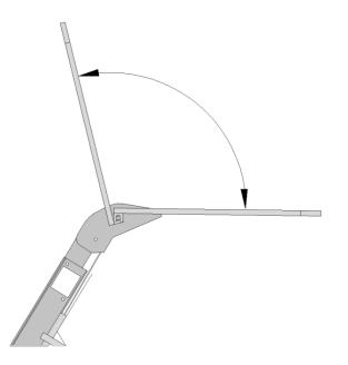
**9.** Fitting centre prop (10 metre machine only). Hook centre prop over prop rest on machine then push up adjust with lever until prop is vertical with machine straight. Prop is self-locking when extended, however lever must be lifted to retract.
