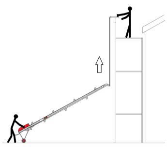
**7.** Once the machine head is on the scaffold, the stand can be positioned and fixed either to the scaffold boards or roof. (Fig. 5.) Alternatively the head can be clamped to the handrail using the clamp provided. (Fig. 6.) Ensure returning belt carriers clear scaffold before starting machine.
